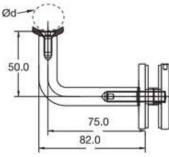
Mounting type: Glass Bore diameter Glass: 16mm Packaging unit: 6 pcs. Usage: Outdoor / Indoor Product shape: Round Reception shape: Round Product diameter: Ø14 mm Reception diameter 3 x options: Ø42,4mm – Ø48,3mm - Plane Glass thickness: 8 – 31,52 mm Material: Stainless steel 304 Surface: Satin Height: 50 mm Width: 82 mm Bore diameter reception side Ø5,5 mm Glass structure: Laminated/monolithic
